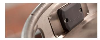
When the application is too demanding for adhesives, but the metal surface cannot be punched for screw or rivet fixing, welding the tag with special bracket is an option for attachment. Welding bracket is made of stainless steel and delivered ready attached to tag with pop rivets. Bracket design allows attachment on both flat and curved surfaces.
